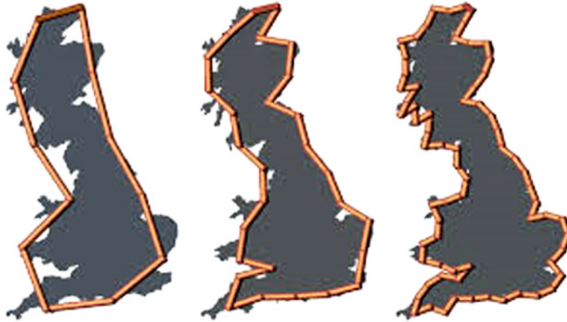
Fig. 7. Unsuccessful traditional technique of determination of the length of Britain coastline. 11.5 sticks of length 200 km gives 2300 km (left side), 28 sticks of length 100 km gives 2800 km (centre), and 70 sticks of length 50 km gives 3500 km (right side)
