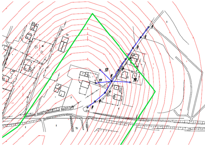
Fig. 5. Forecast trough of subsidence caused by exploitation of the W-5 longwall with marked location of the terrain line (Source: Material prepared by the Marcel Coal Mine)
